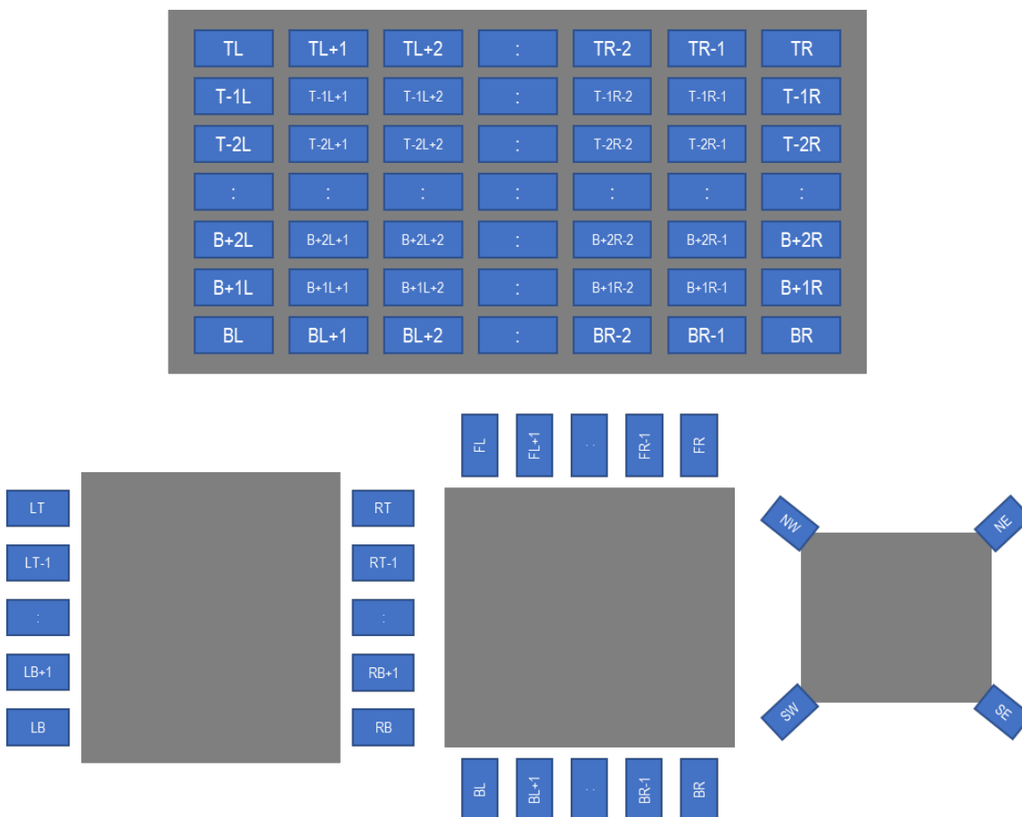
Figure 11 – Terminal Numbering Pattern Samples
